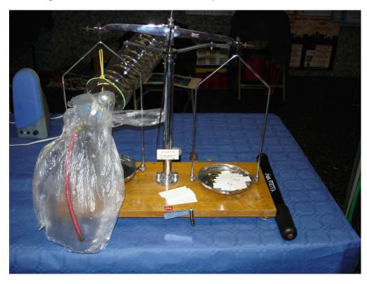
To equilibrate the balance again, just remove the small paper sheets that were used to determine the mass of the air litre introduced into the bottle. The Archimedean buoyant force is then equal to the weight of the air that was moved.
